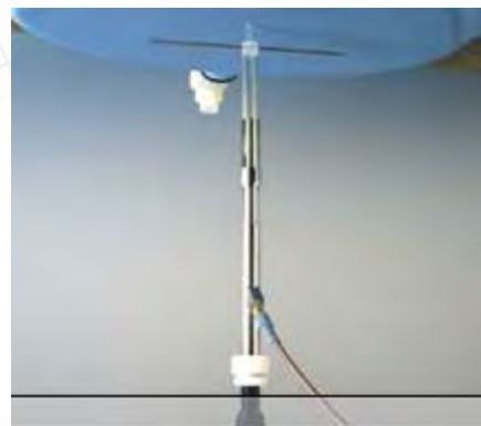
Photograph of the dipole Antenna
