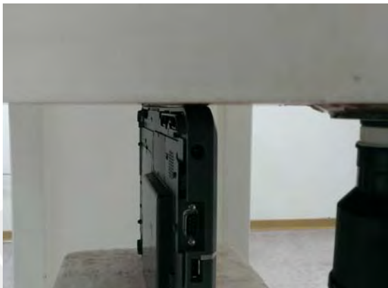
Fig.10 EUT Bottom side with optional battery to flat phantom
