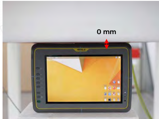
Fig.9 EUT Bottom side to flat phantom
