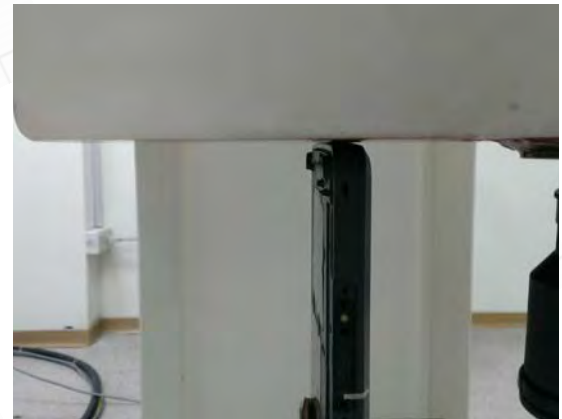
Fig.12 EUT Left side to flat phantom
