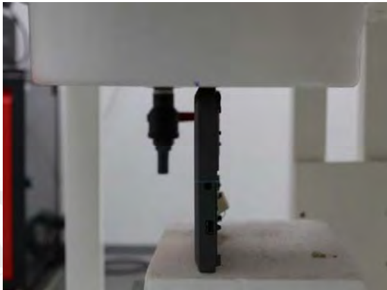
Fig.9 EUT Bottom side to flat phantom
