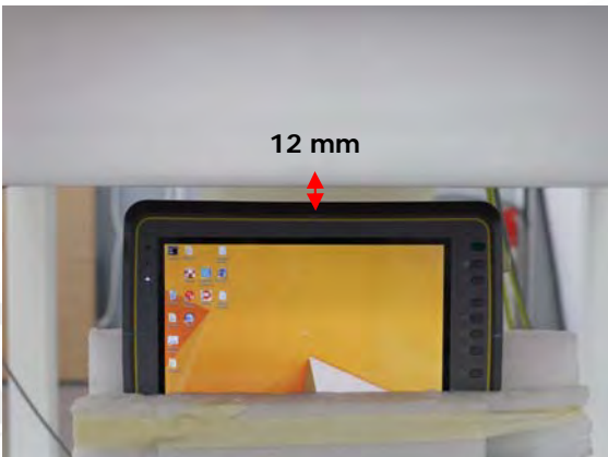
Fig.6 EUT Top side (12mm) to flat phantom
