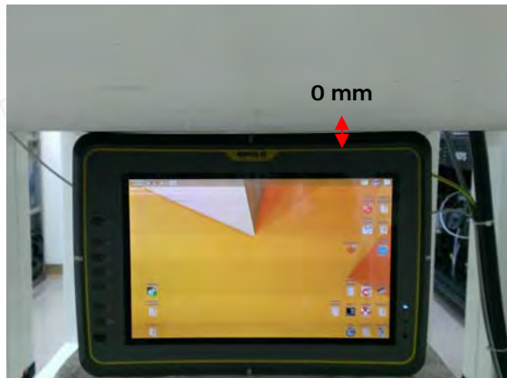
Fig.10 EUT Bottom side with optional battery to flat phantom
