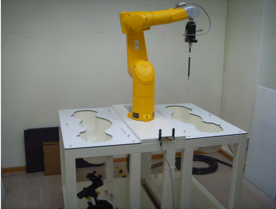
Fig.1 Photograph of the SAR measurement system
