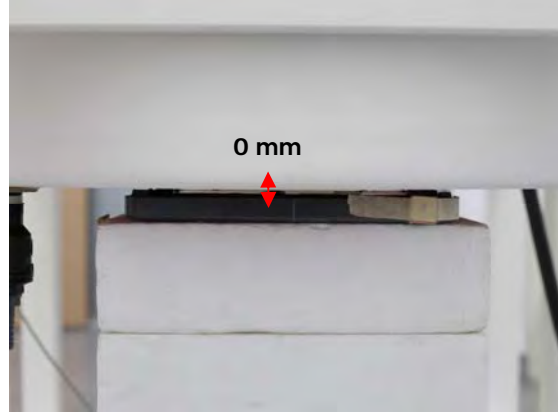
Fig.3 EUT Back side to flat phantom
