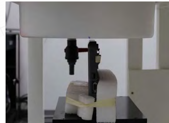
Fig.6 EUT Top side (12mm) to flat phantom
