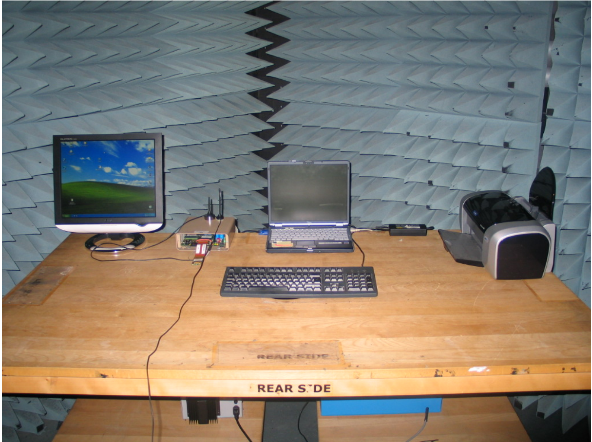
Photo 1: Test setup for radiated measurements
