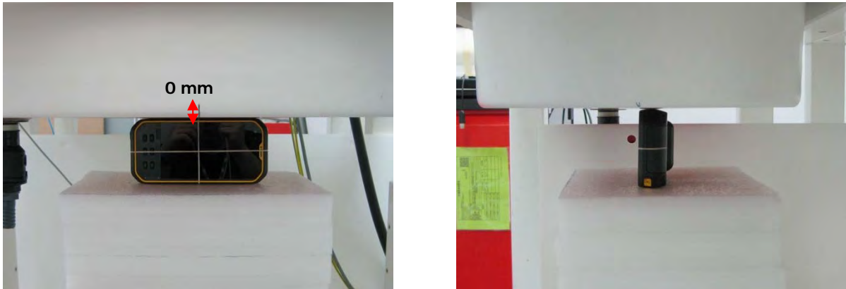
Fig.9 EUT Left side to flat phantom
