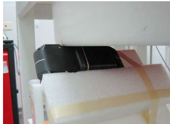
Fig.4 EUT Back side (WLAN Main) to flat phantom
