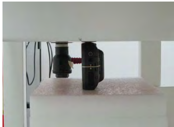
Fig.8 EUT Right side to flat phantom
