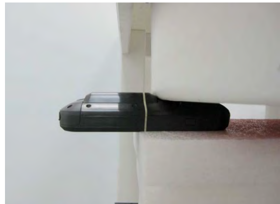
Fig.5 EUT Back side (WLAN Aux) to flat phantom
