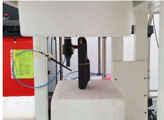
Fig.6 EUT Top side to flat phantom
