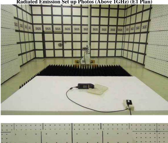
Radiated Emission Set up Photos (Above 1GHz) (E1 Plan)
