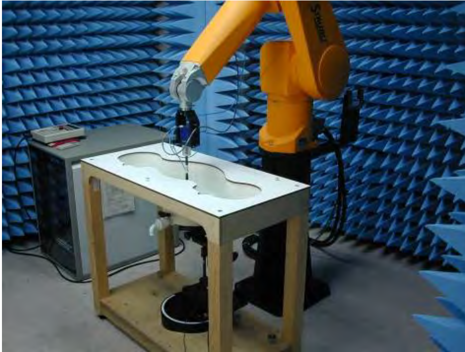
Fig.1 Photograph of the SAR Measurement System
