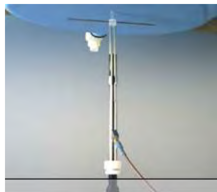
Photograph of the Dipole Antenna
