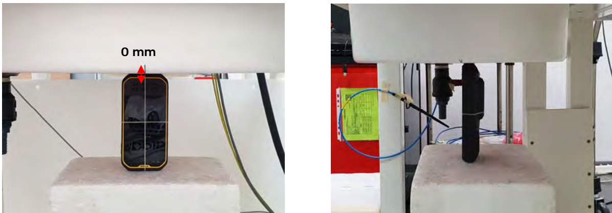
Fig.8 EUT Bottom side to flat phantom
