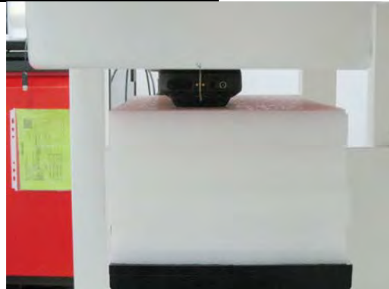
Fig.3 EUT Front side to flat phantom
