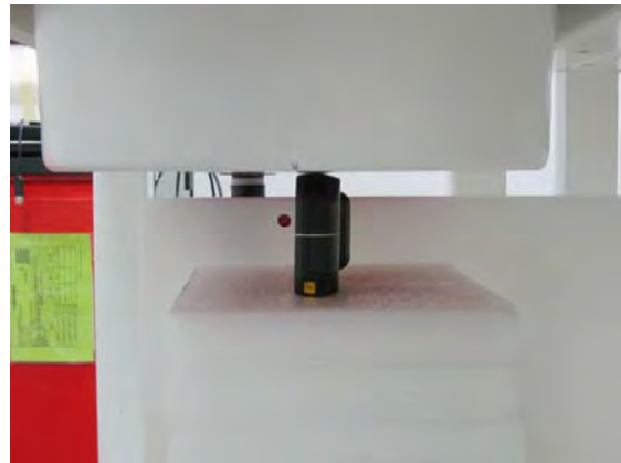
Fig.10 EUT Left side to flat phantom
