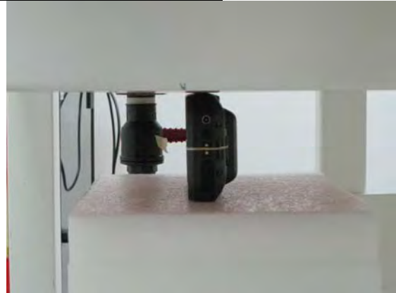
Fig.9 EUT Right side to flat phantom
