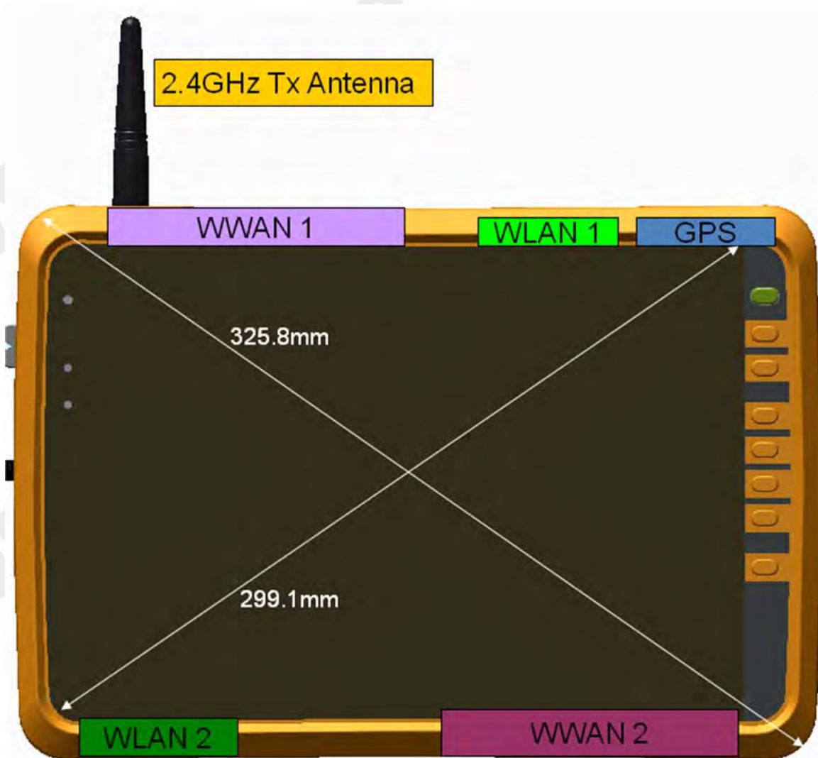
Front view of the tablet with transceiver attached
