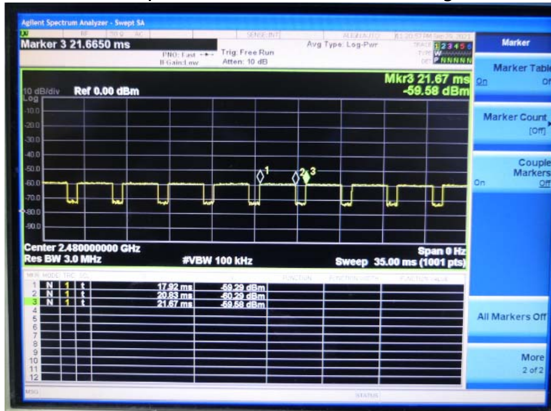
Time-domain plot for Bluetooth transmission signal
