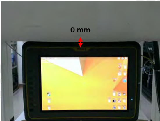
Fig.11 EUT Bottom side with transceiver to flat phantom
