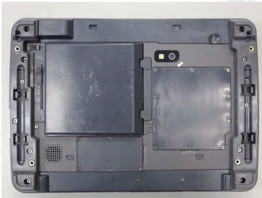
Fig.17 Back view of EUT with bumper and optional battery
