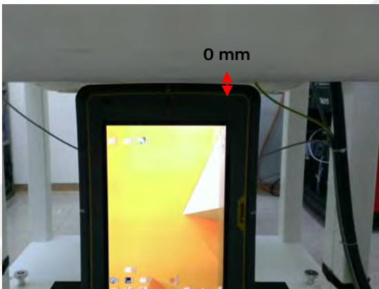
Fig.13 EUT Right side to flat phantom
