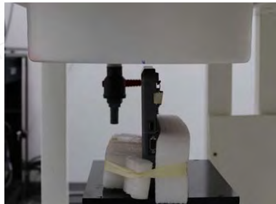
Fig.6 EUT Top side (12mm) to flat phantom
