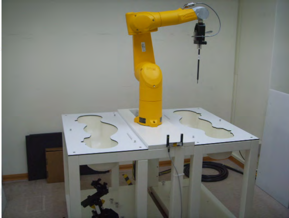
Fig.1 Photograph of the SAR measurement system
