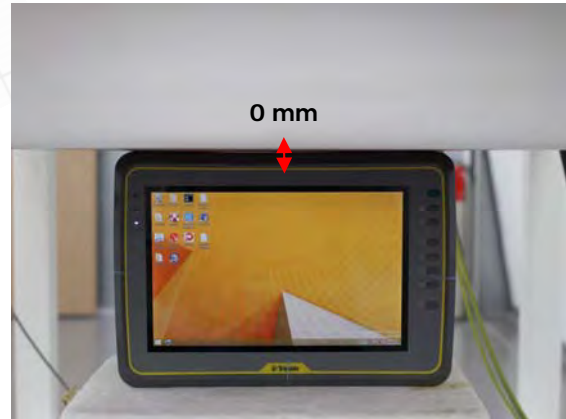
Fig.5 EUT Top side to flat phantom
