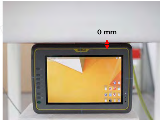
Fig.9 EUT Bottom side to flat phantom
