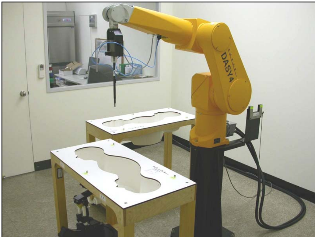
Fig. 5 The DASY4 System used in ETC set-up with two phantoms
