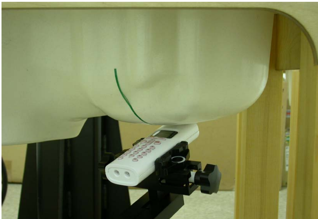
Measurement Position of Left-Tilt (LT) with Handset
