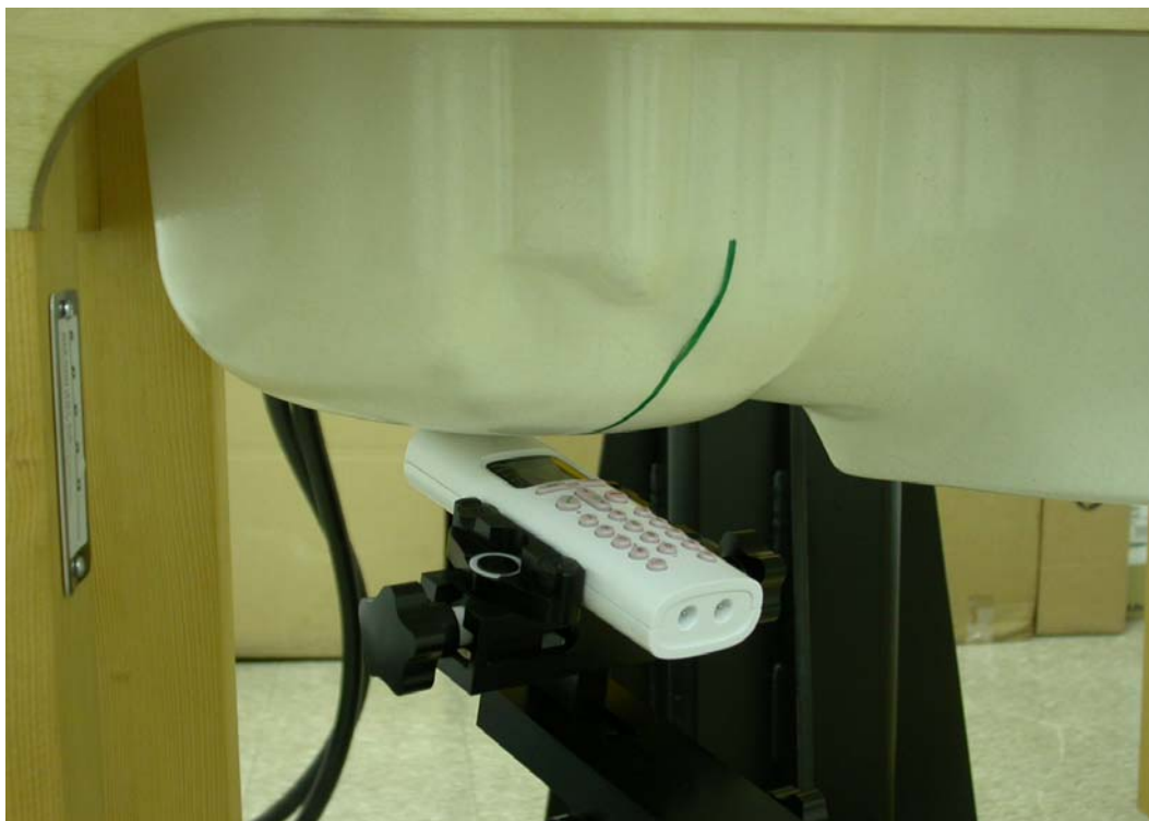
Measurement Position of Right-Tilt (RT) with Handset
