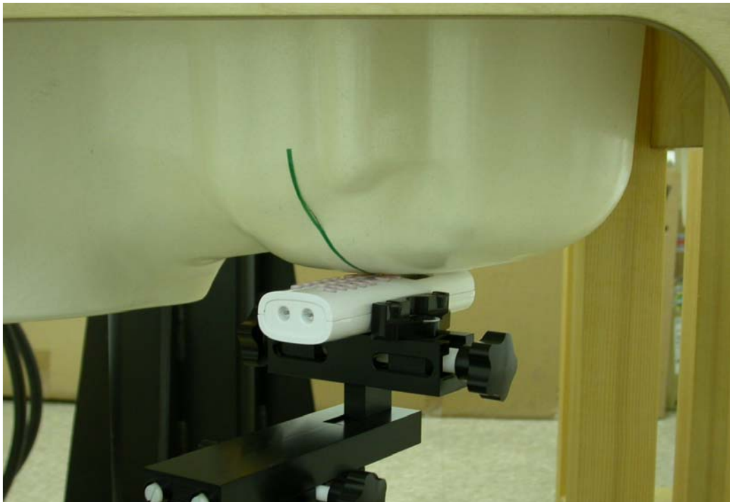
Measurement Position of Left-Cheek (LC) with Handset
