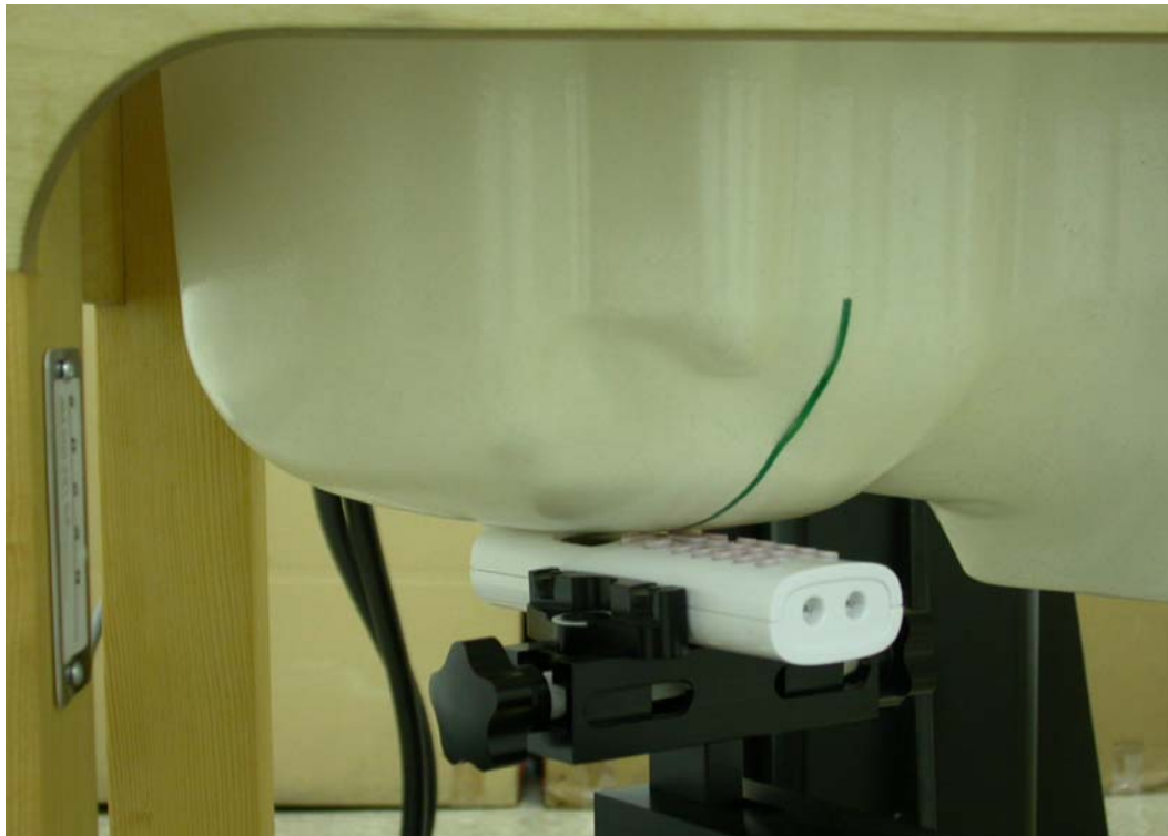
Measurement Position of Right-Cheek (RC) with Handset
