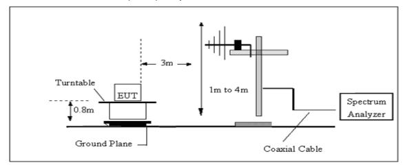
(B) Radiated Emission Test-Up Frequency Above 1GHz
