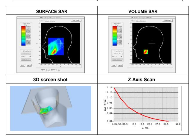
Plot 6: DUT: 5.5inch Smart phone; EUT Model: G25523K
