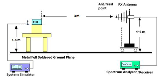
For radiated test from above 1GHz
