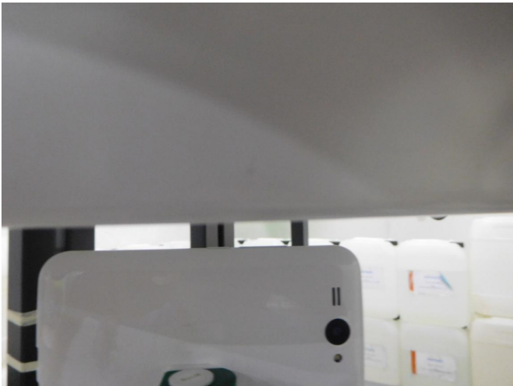
Body right side(separation distance is 10mm)
