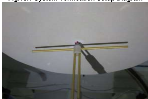
Fig.10.2 Photo of Dipole setup
