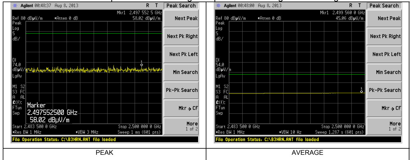
Screen Capture Demonstrating Compliance at the Higher Band-Edge
