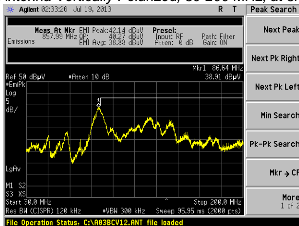
Antenna Vertically Polarized, 30-200 MHz, at 3m
