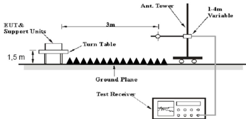
The radiated emission tests were performed in the 3 meters chamber test site, using the setup accordance with the ANSI C63.10-2013. The specification used was the FCC 15.209, and FCC 15.247 limits. The external I/O cables were draped along the test table and formed a bundle 30 to 40 cm long in the middle.
