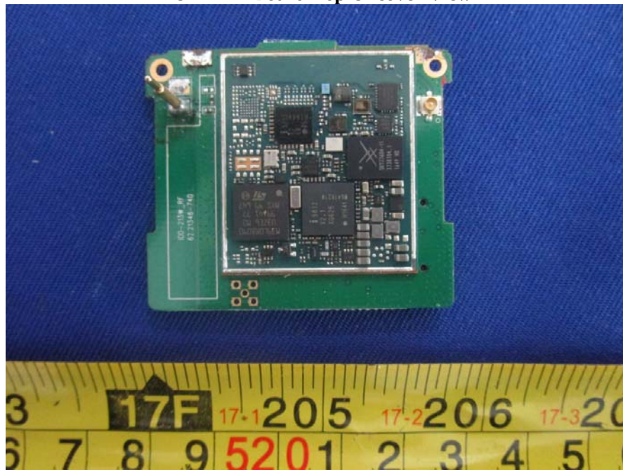
EUT – RF Board Top Uncover View
