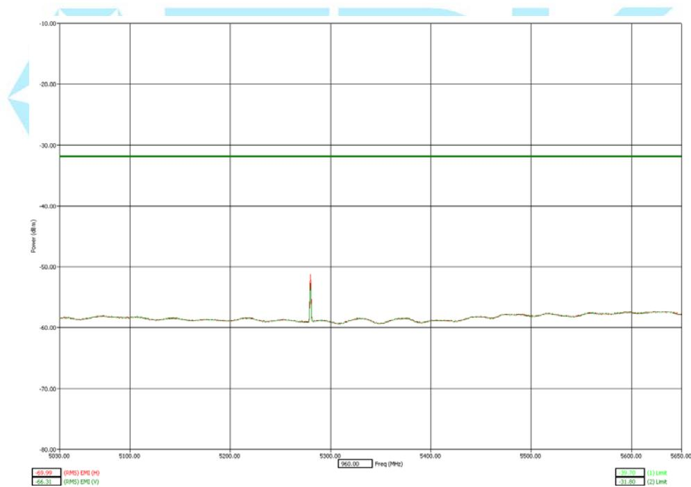
Measurements made with 1 MHz RBW / 3 MHz VBW at 1 meter distance
