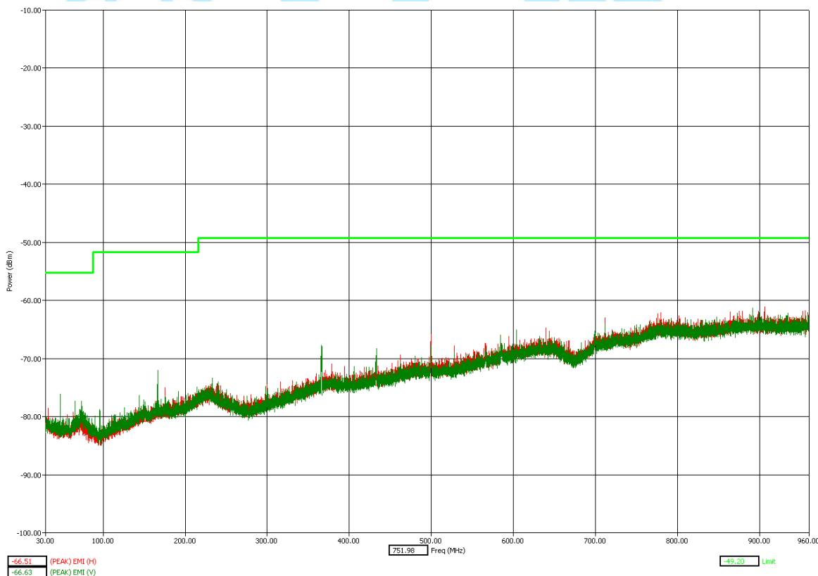
All digital emissions from the transmitter whether radiating from the antenna port or not intended to be radiated from the antenna port meet the limits of 47 CFR, Part 15, Subpart F, §15.519(c) (§15.209).
