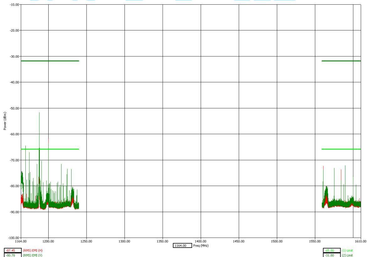
Lower limit line is 47 CFR, Part 15 subpart F
