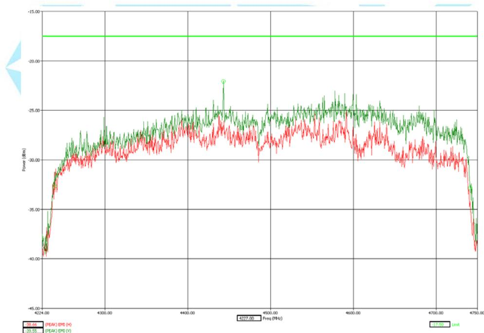
Measurements made with Peak detector, RBW = 8 MHz, VBW = 8 MHz, Measurement Time = Auto, Measurement distance = 3 m, Antenna bore-sighted to EUT and maximized in azimuth and elevation.
