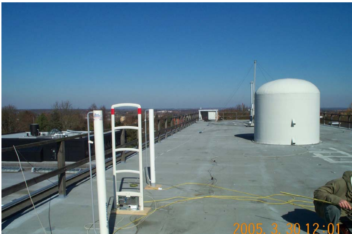
Photo 4 Radiated emission. 30 m OATS.
