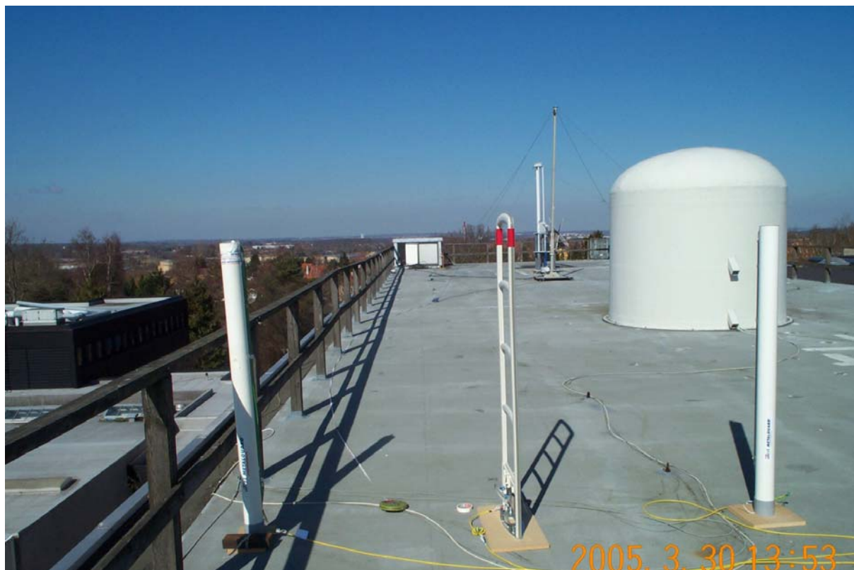
Photo 5 Radiated emission. 30 m OATS.
