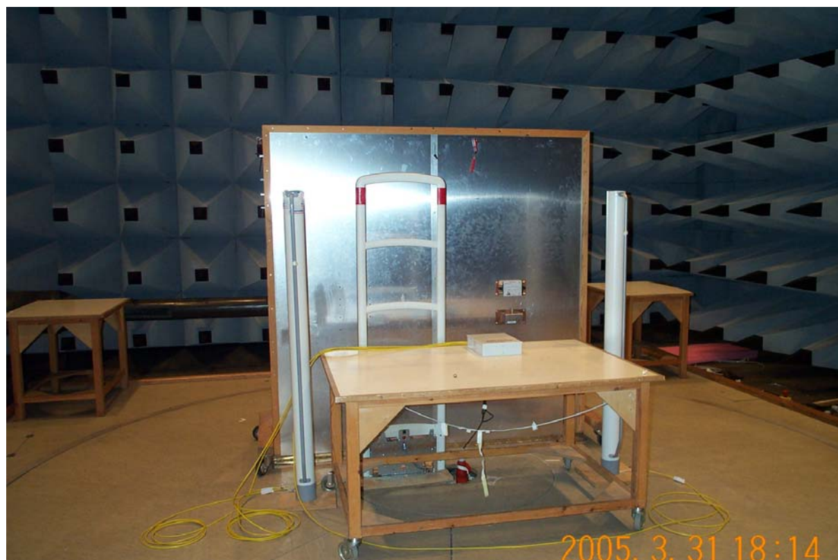
Photo 3 Conducted emission, 0.15 - 30 MHz.
