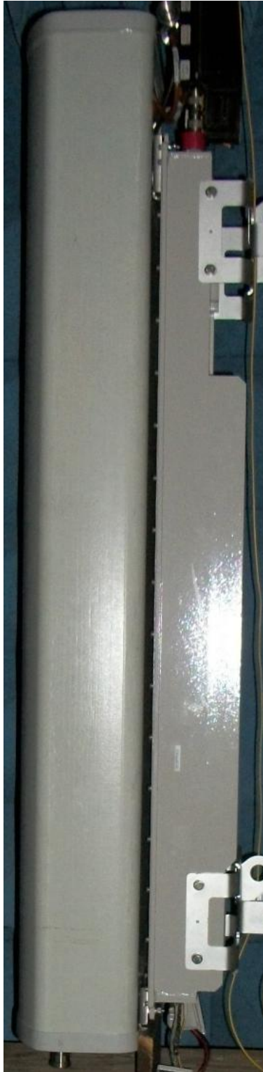
RRH 2x45W 1900MHz RF151032 with antenna assembly
