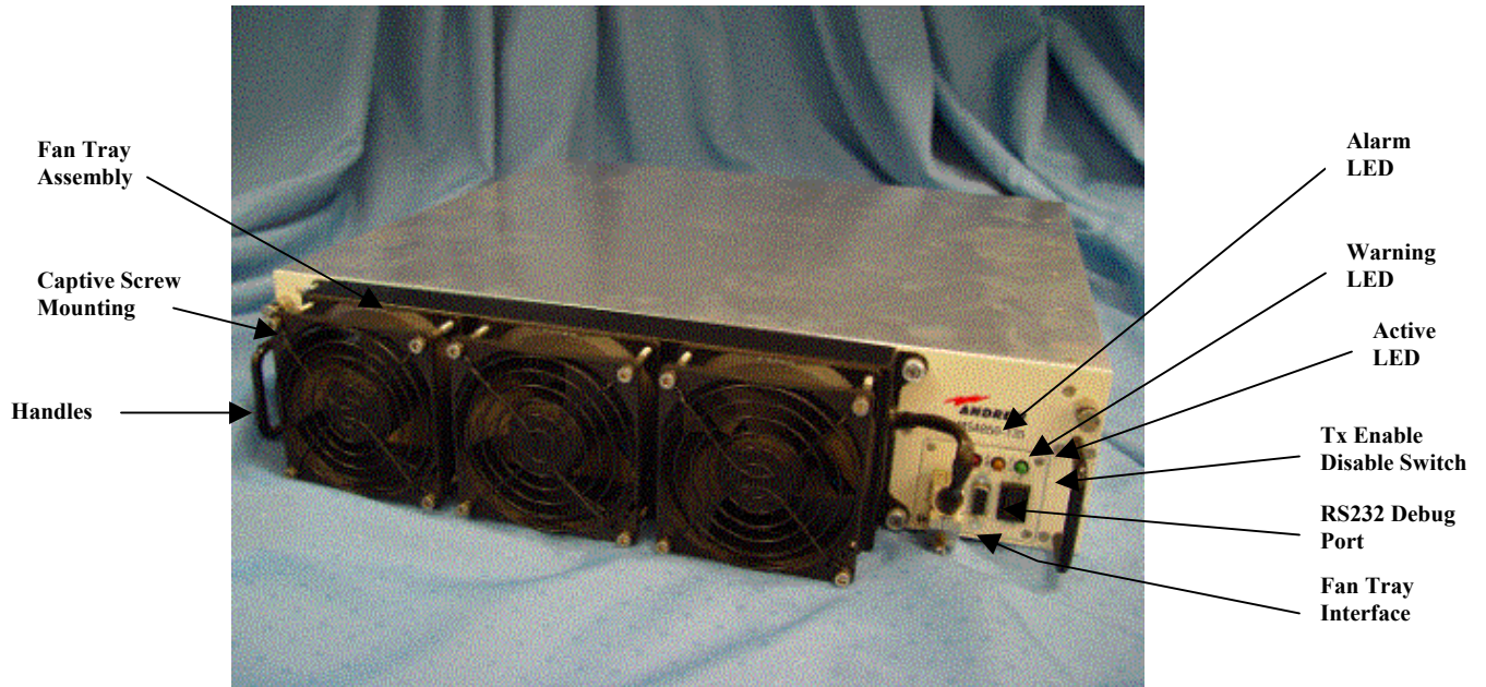
Figure 3 MSA850-135 MCPA Front Panel
