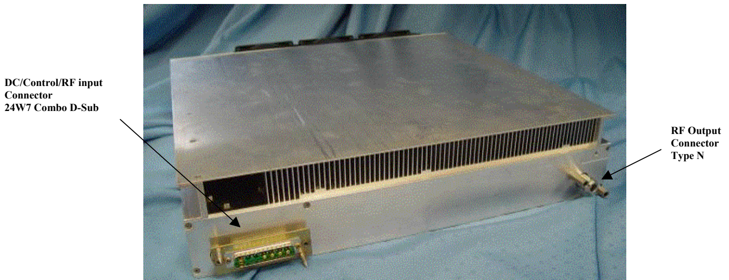
Figure 2 MSA1900-135 Rear Panel
