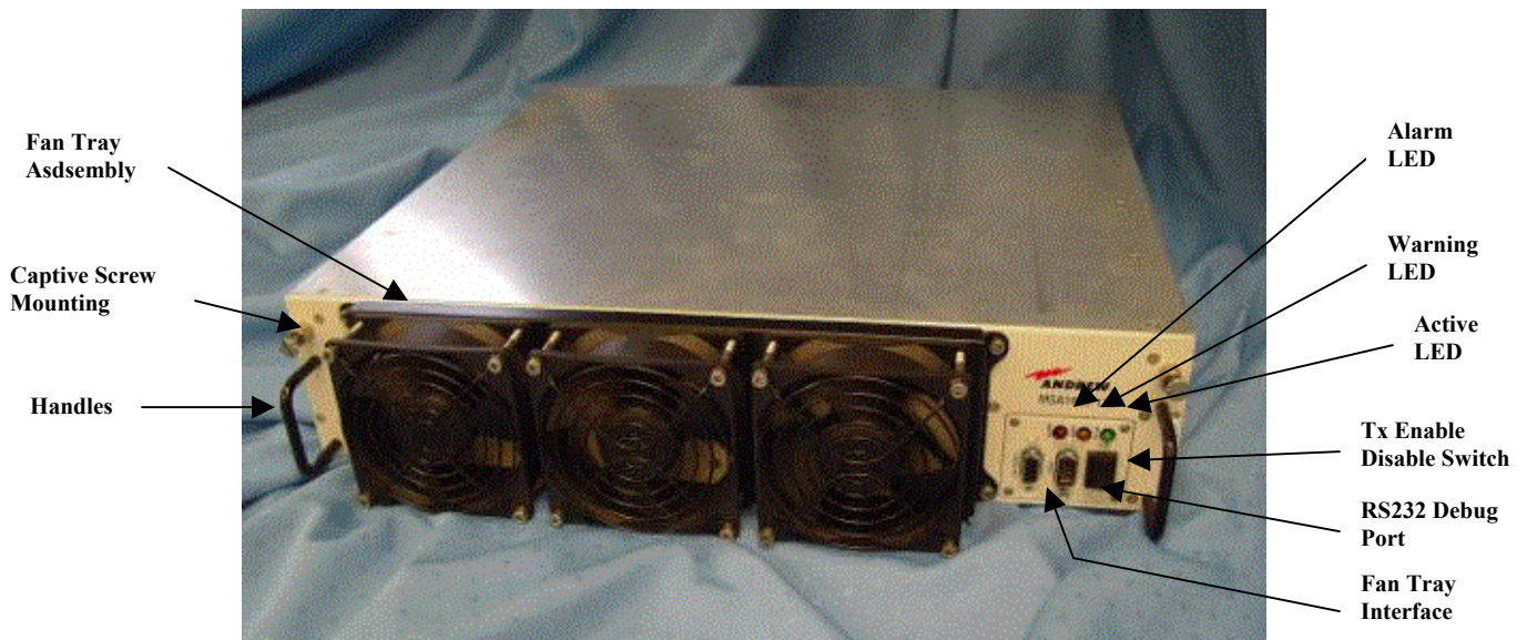
Figure 1 MSA1900-135 MCPA Front Panel
