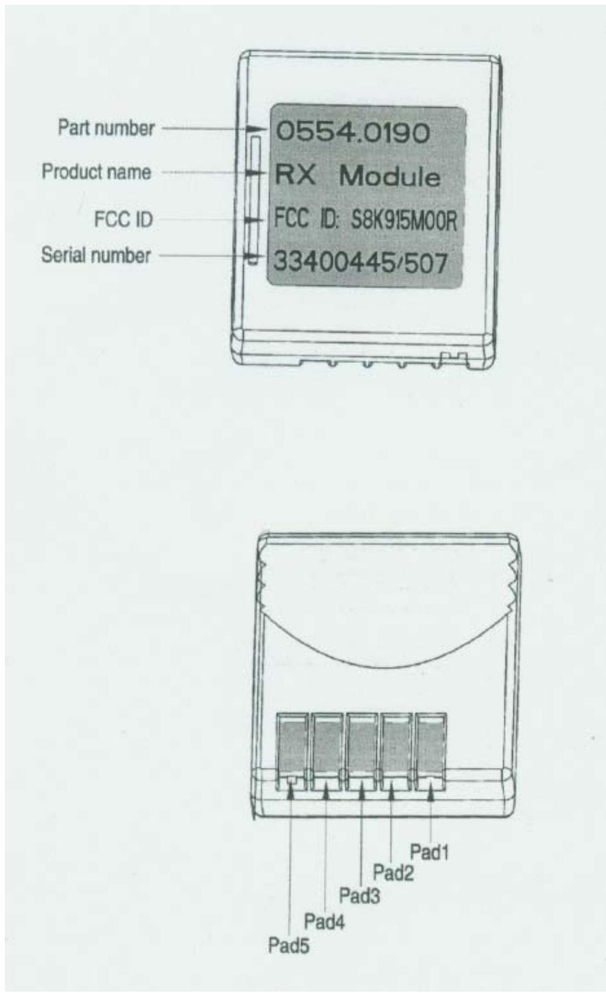
The FCC label is stucked on the surface of the receiver module. This module can be accessed by the end user by removing the cover of the module compartment. User is required to install the receiver module on the instrument in order to activate the receiving function.
