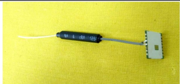
Module+Antenna – Back photo The antenna is welded on the module.
