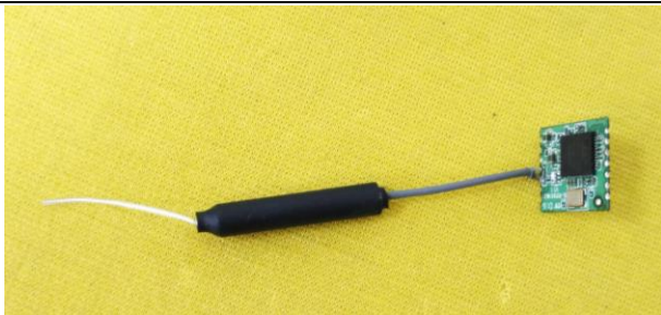
Module+Antenna – Front photo The antenna is welded on the module.
