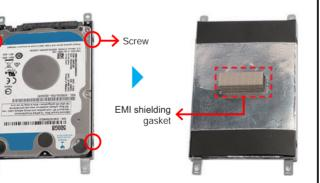
2. Tear off the adhesive tape of the serial ATA and power
