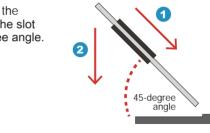
4. Carefully push down the memory module until it snaps into the locking mechanism.
