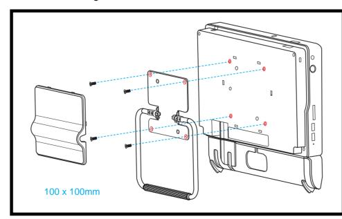
If you are mounting your P20U to the wall, remove the cover on the back of the P20U first. Unscrew four screws of the stand mount and remove the stand. The VESA standard lets users mount it on to walls easily. Please refer to the user guide of the wall/arm mount kit you bought separately to install it.
