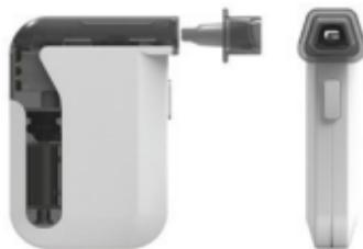
**Step 1.** If you would like to use a mouthpiece, attach it to the BACtrack Mobile. Note: Using a mouthpiece is optional and does not affect the performance of the breathalyzer; however it does provide a hygienic way to test others.
