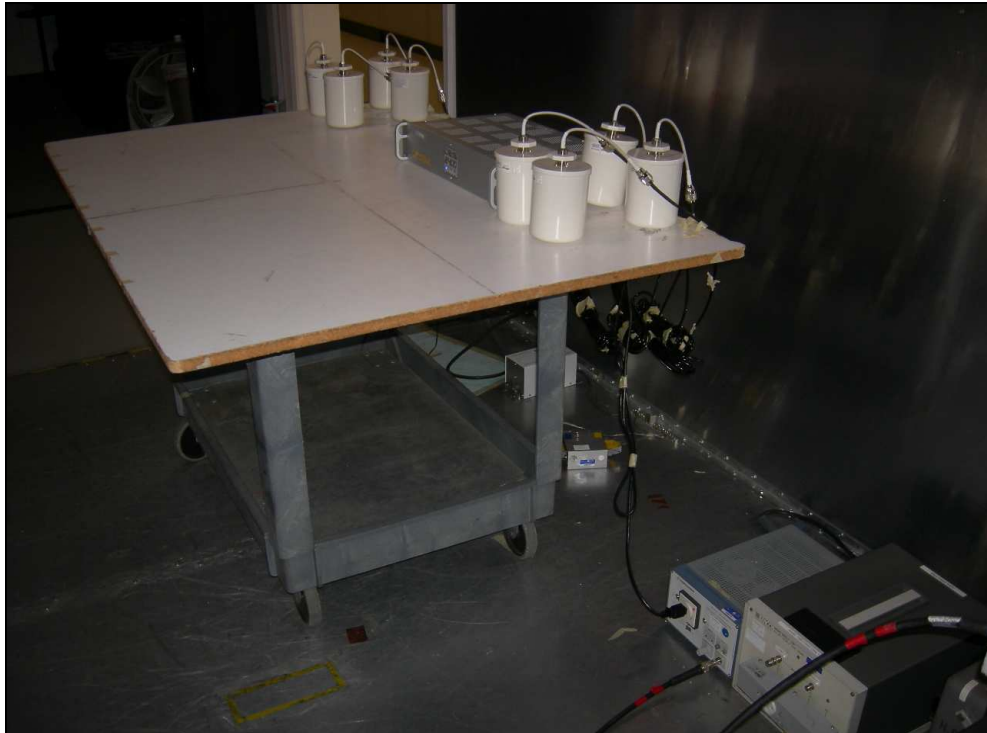
Figure 10: Conducted Emissions – DAS2400
