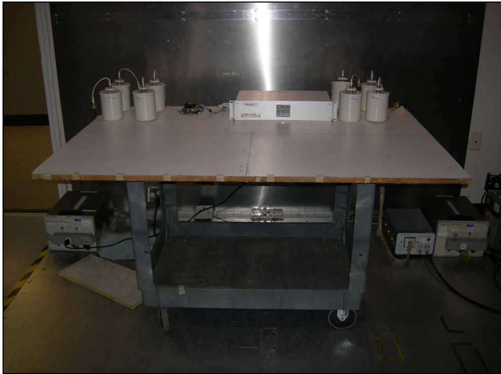
Figure 11: Conducted Emissions – DAS2400 Supply
