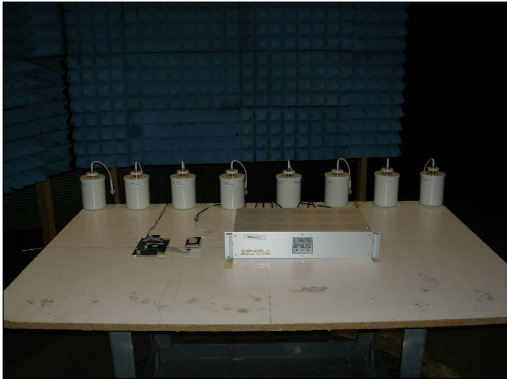
Figure 7: Radiated Emissions – Ceiling Antenna XPOS
