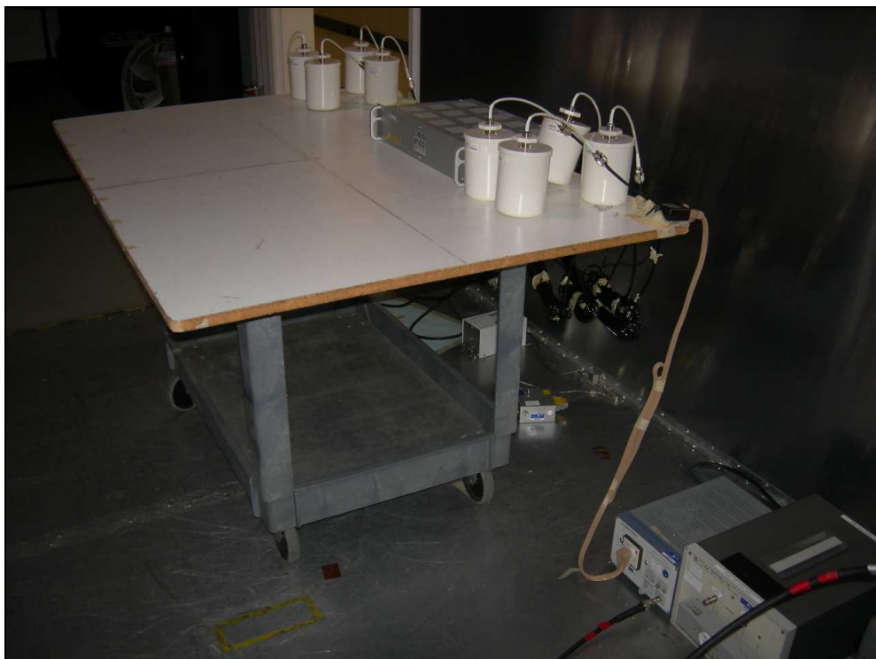
Figure 12: Conducted Emissions – DAS2400 Supply
