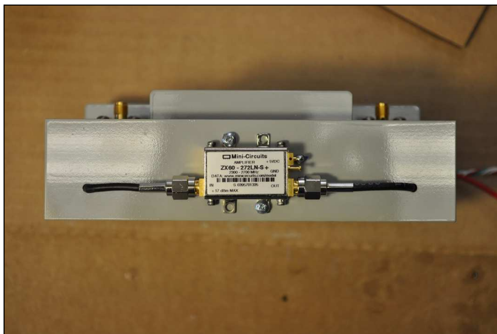
Figure 3: Internal Photo – Side View of RF Amplifier
