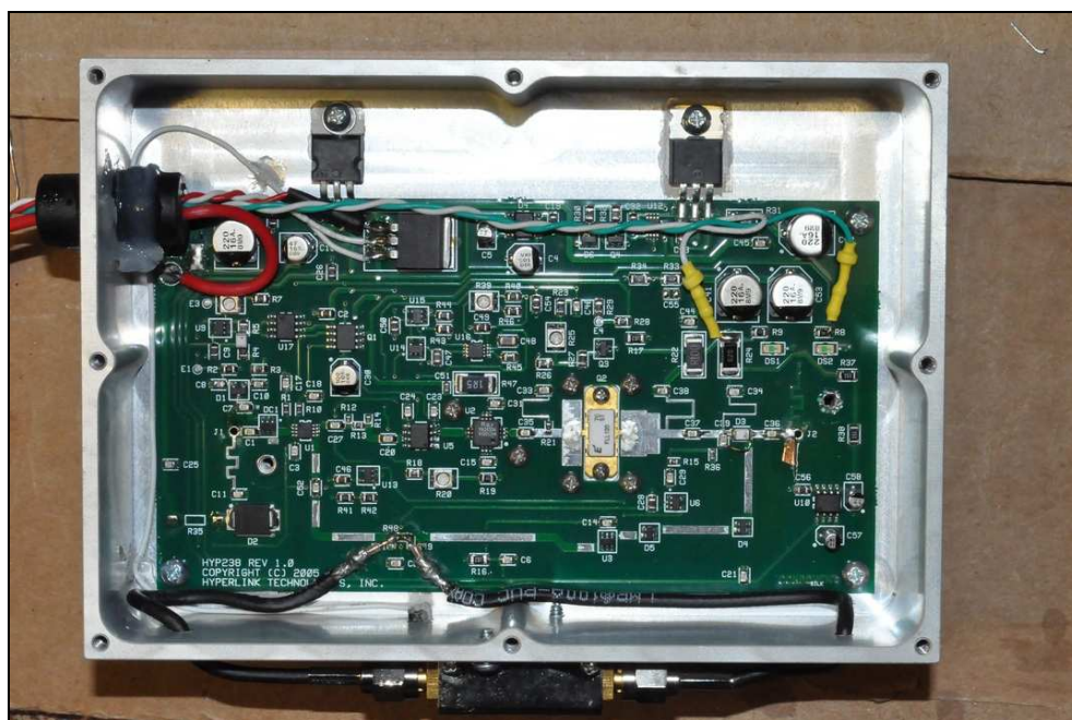
Figure 4: Internal Photo – RF Amplifier Board installed in Amp Chassis
