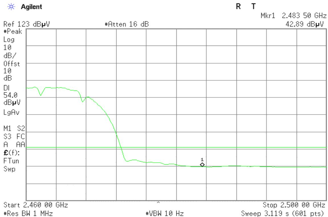
**Band Edges (IEEE 802.11g / CH Low)****Detector mode: Peak****Polarity: Vertical**
