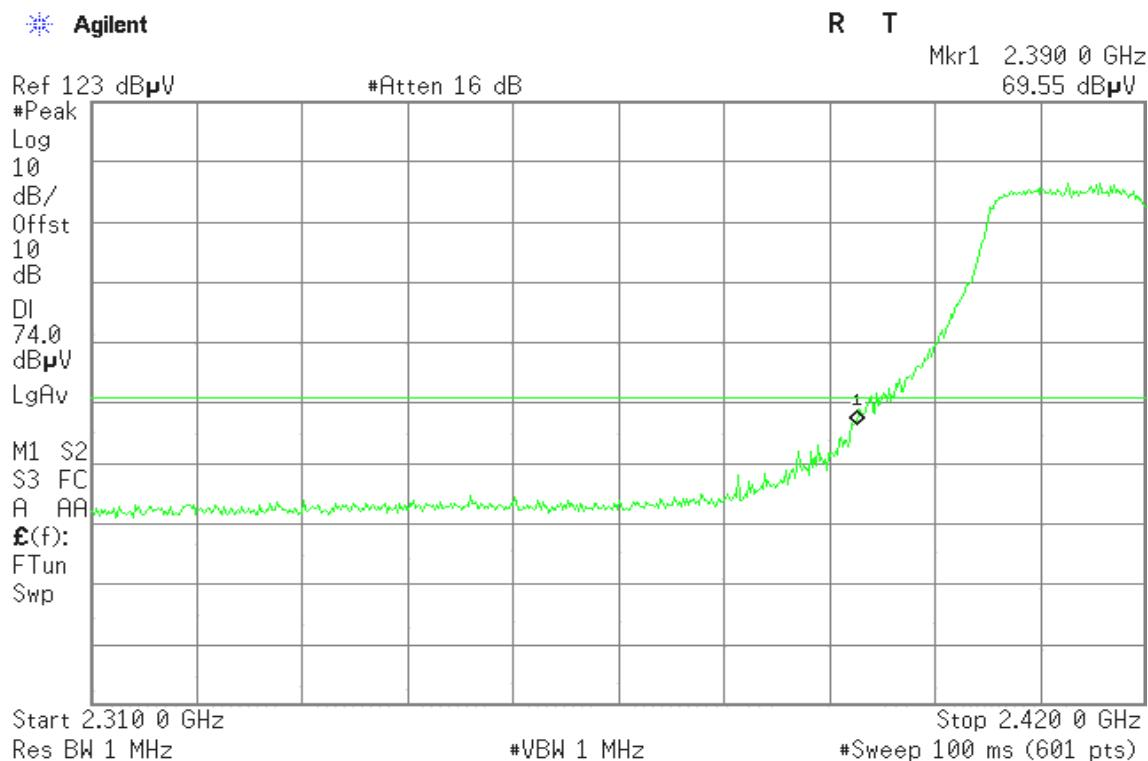
**Detector mode: Average****Polarity: Vertical**
