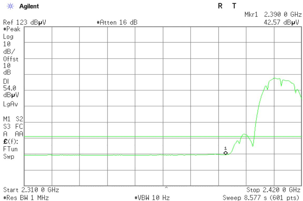
**Band Edges (IEEE 802.11b / CH High)****Detector mode: Peak****Polarity: Vertical**
