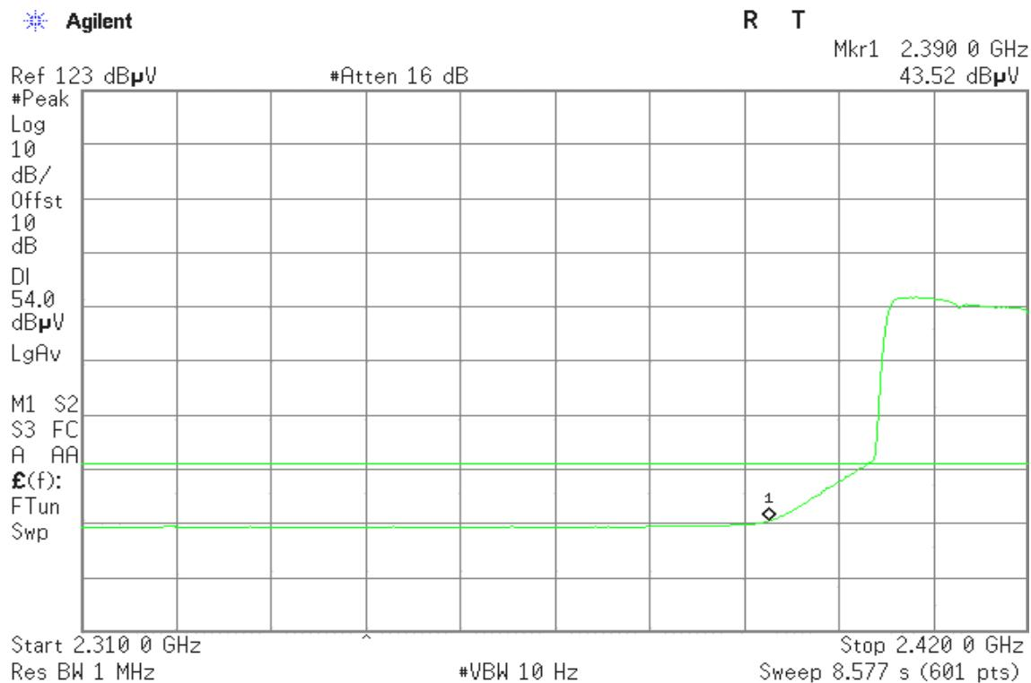
**Band Edges (IEEE 802.11g / CH High)****Detector mode: Peak****Polarity: Vertical**
