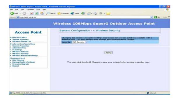
WEP is a basic encryption method, which is not as secure as WPA. To use WEP, you will need to select a default transmit key and a level of WEP encryption,
