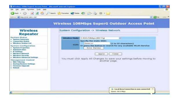
After click on the "Site Survey" button, you can choose the Access Point you need to extend its range by clicking on "BSSID" column. Then "Apply" the change to make sure system working properly with new setting.
