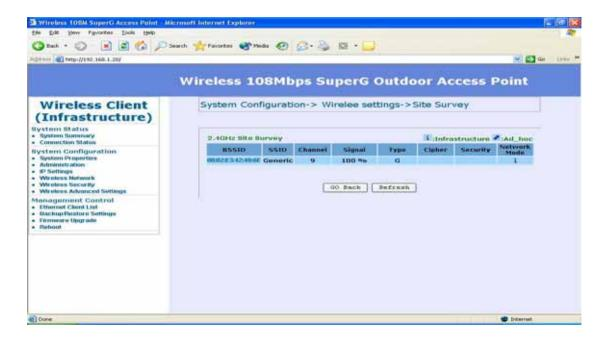
After you determine which AP (SSID) to join, you can click on the BSSID column your want to choose. The system will automatically join the SSID you specified after reboot.
