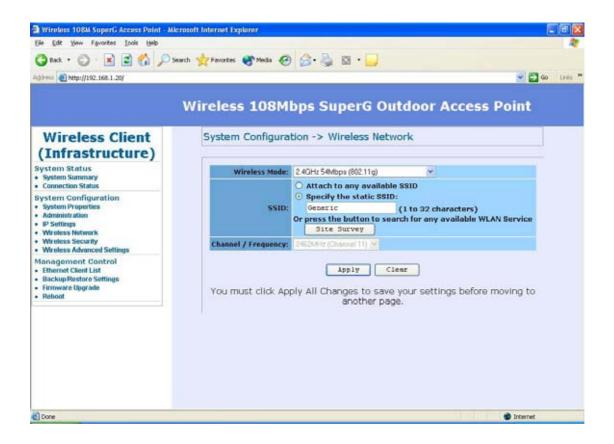
The Site Survey page can help you identify all the APs currently working in your environment. Just easily click on the BSSID column, the system will join you to the SSID you specify. In the Site Survey page you can also see the details of all SSID currently available.
