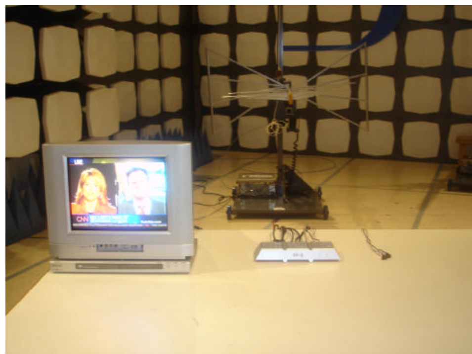
Photograph 3: Set-up for Radiated Emission in Horizontal Orientation
