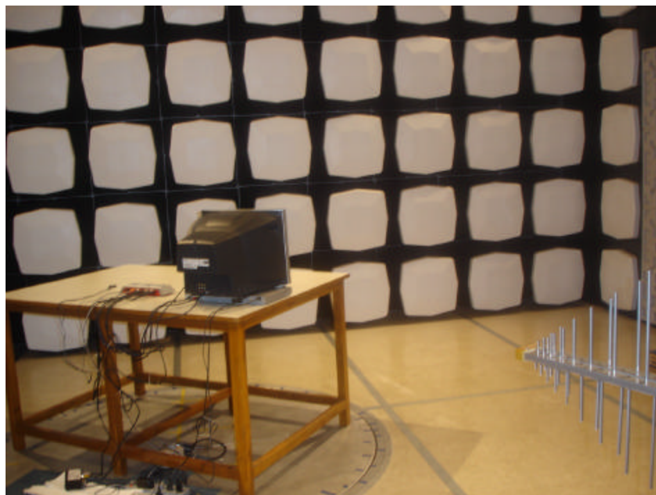
Photograph 2: Set-up for Radiated Emission in Vertical Orientation
