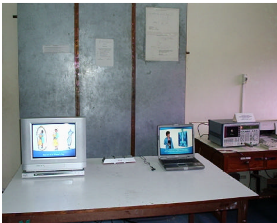
Photograph 1: Set-up for Conducted Emission on AC Mains
