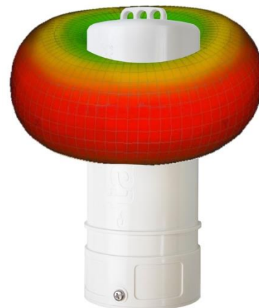
Figure 5 - Internal antenna propagation pattern
