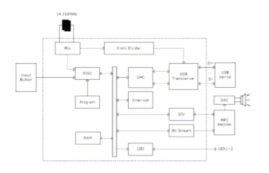
VLSI 1003 is a single-chip solution for an MPEG layer 1,2 and 3 audio decoder. It is receive input bitstream through a serial input bus from the OTI-6888. which it worked slave mode The input stream is decoded control to an 18-bit oversample, multi-bit, sigma-delta DAC. The decoding is controlled via a serial control bus, after decoded, stereo audio signal be amplified and send to the FM circuit.
