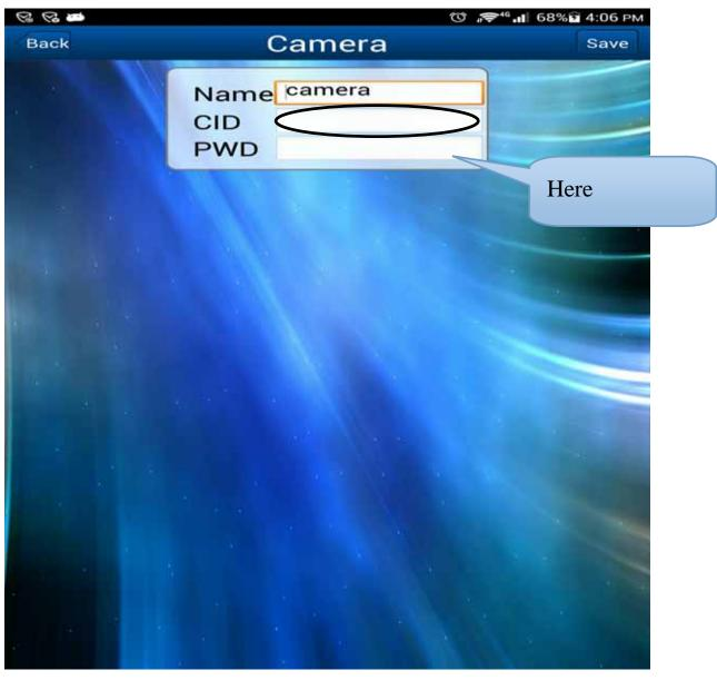
You can enter a desired NetCamera name (e.g., 28 shown above) on the top field. You will also need to enter the CID and PWD of the NetCamera that you had previously copied down here on this menu to complete the customization process.
