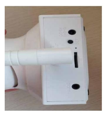
Note: the Audio port is for connecting to external speakers if needed. The NetCamera already has build-in speakers.
