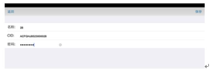
Enter previously saved CID name and Passcode of the saved NetCamera, and a camera name that better reflect its location onto corresponding entry field to complete NetCamera registration in the APP. A newly added NetCamera name should show up in the APP camera list as shown in the picture below
