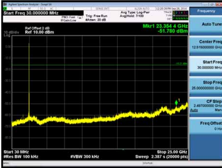
Test Model PSD(Power Spectral Density ) RBW=100kHz Bluetooth 4.0 DTS Channel 19: 2480MHz
