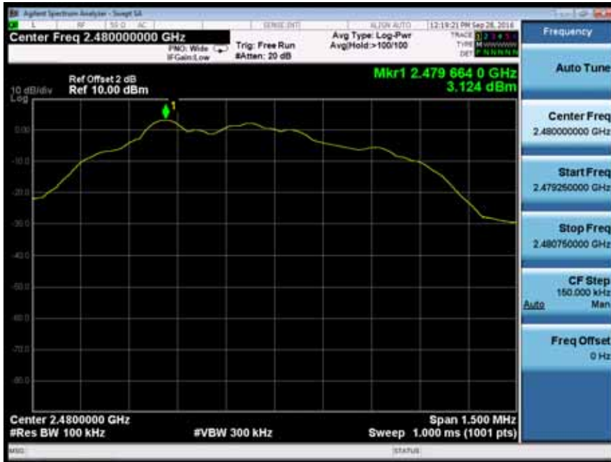
Test Model PSD(Power Spectral Density ) RBW=100kHz Bluetooth 4.0 DTS Channel 19: 2480MHz
