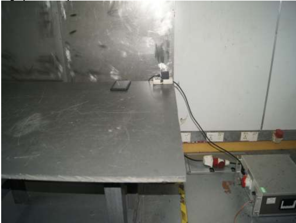
Photograph 2: Set-up for Spurious Emissions for below 30MHz
