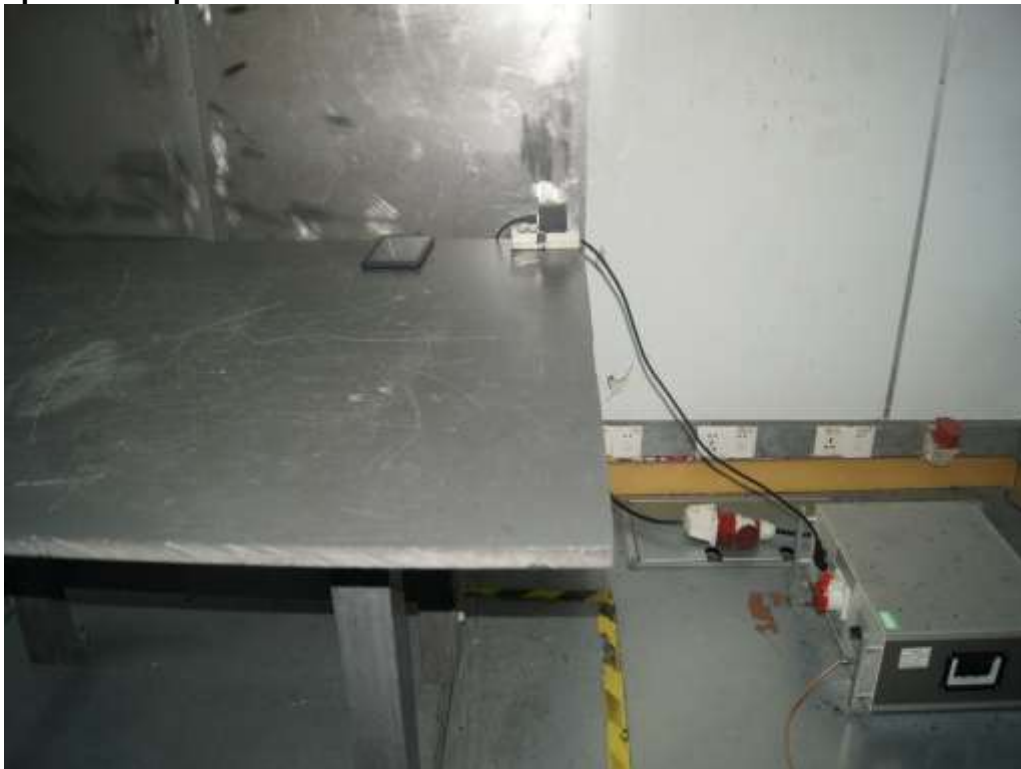
Photograph 2: Set-up for Radiated Emission of below 1GHz
