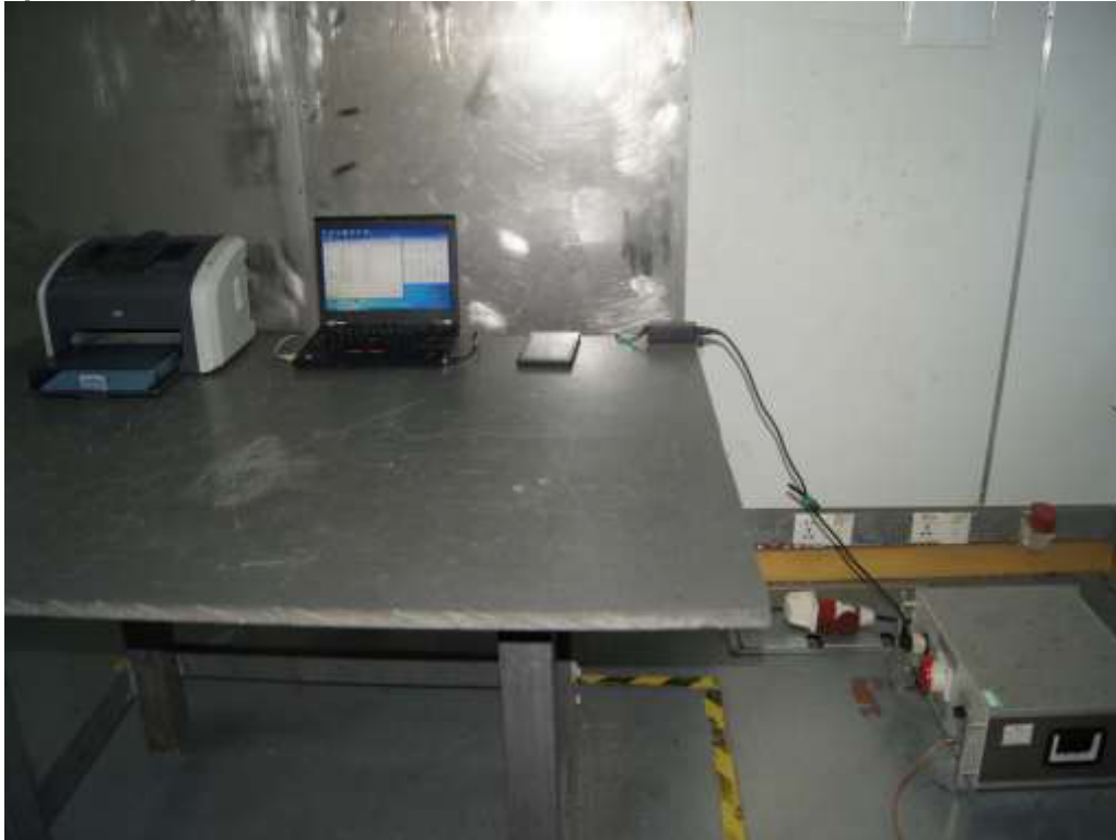
Photograph 2: Set-up for Radiated Emission of below 1GHz
