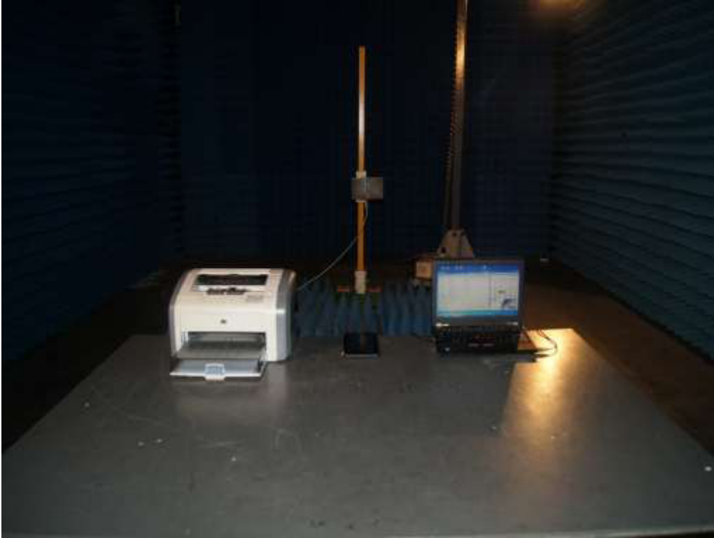
Photograph 4: Set-up for Radiated Emission of 18 - 25GHz
