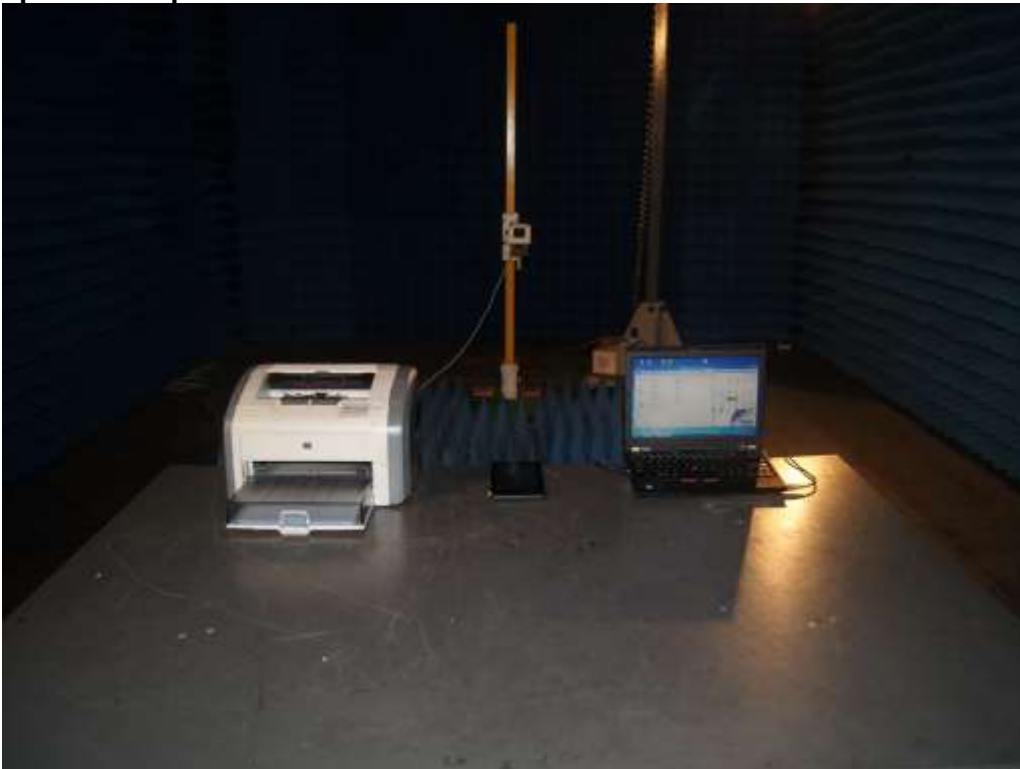
Photograph 4: Set-up for Radiated Emission of 18 - 25GHz
