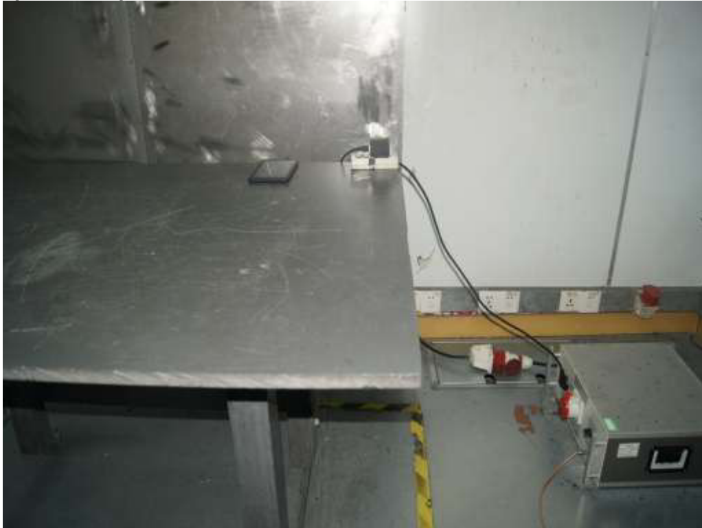
Photograph 2: Set-up for Radiated Emission of below 1GHz
