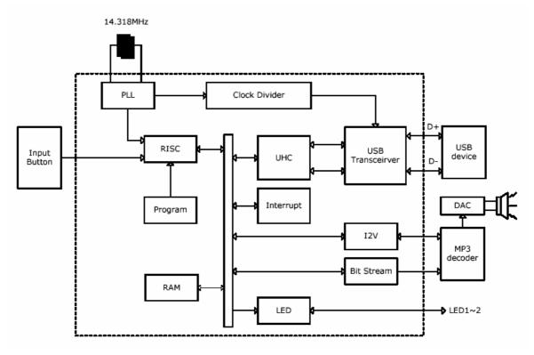
OTi-001316V01 is a single-chip solution for an MPEG layer 1, 2 and 3 audio decoder. The chip contains a high-performance low-power DSP processor core (OTI\_DSP), working memory, 4
