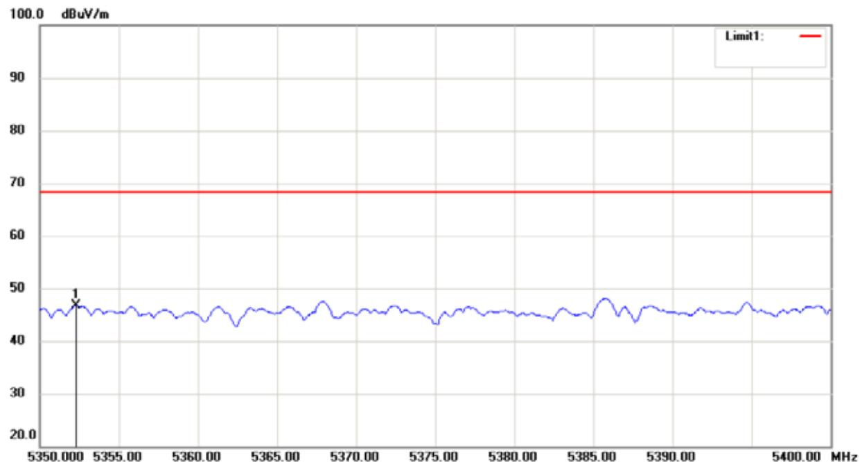
■  For Undesirable radiated Spurious Emission in UNII Band II-A
