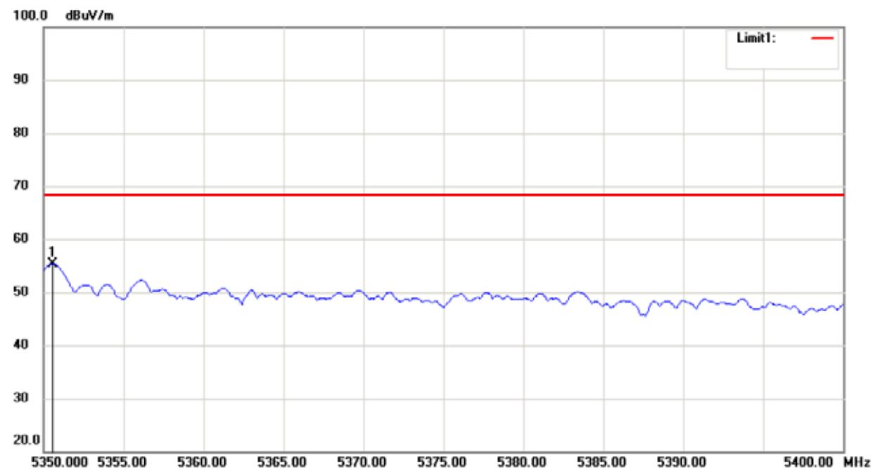
■  For Undesirable radiated Spurious Emission in UNII Band II-C
