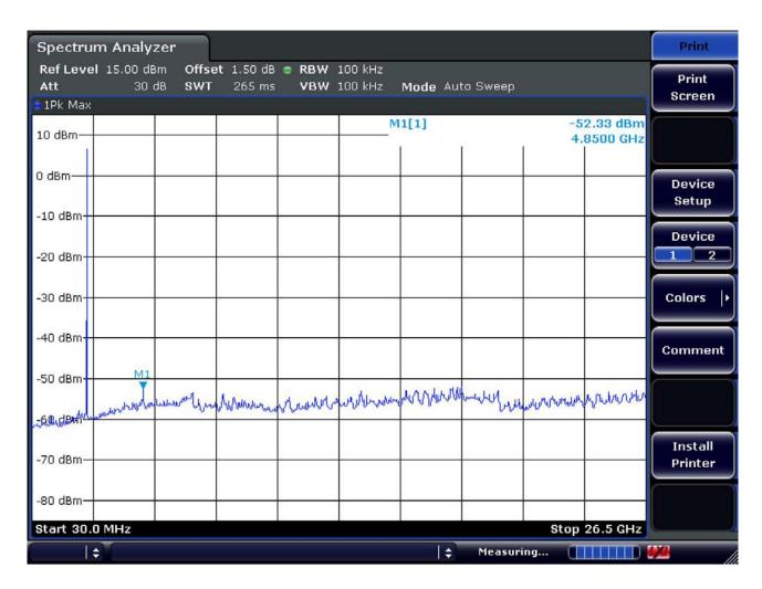
$\label{eq:midchannel} Mid \ channel$   $Frequency \ Range = 30 \ MHz \sim 10^{th} \ harmonic.$
