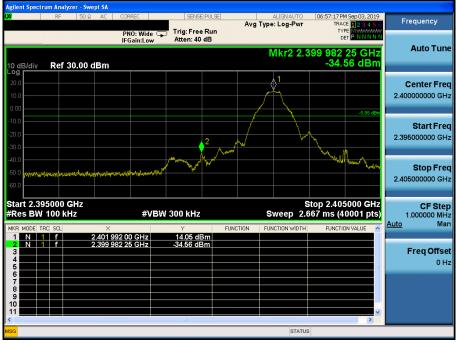
Low Band-edge <u>Hopping mode & Modulation : GFSK</u>
