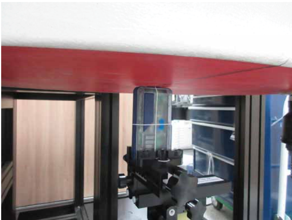
Bottom from Flat Phantom Ant. Folded (Separation Distance: 0 cm)
