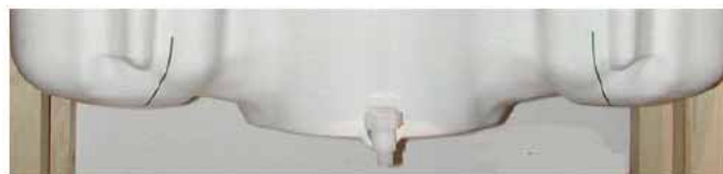
Figure 7.2 SAM Twin Phantom shell
