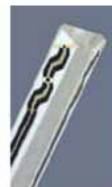
Figure 3.3 Probe Thick-Film Technique
