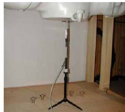
Figure 12.1 Dipole Validation Test Setup
